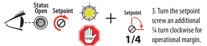
3. Turn the setpoint screw an additional 1/4 turn clockwise for operational margin.
