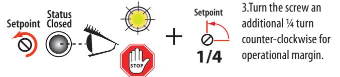
3. Turn the screw an additional 1/4 turn counter-clockwise for operational margin.
